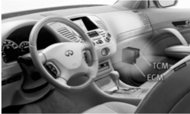
It tailors the engine operation by controlling fuel injection amount and timing, plus ignition timing. ECCS monitors:
