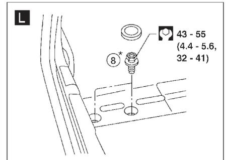
\* : Bumper assembly mounting bolts, screws, nuts, and clips
