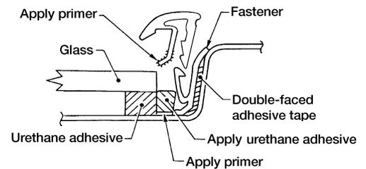
4. Install molding by aligning the molding mark located on center with vehicle center. Be sure to install tightly so that there is no gap around the corner.
