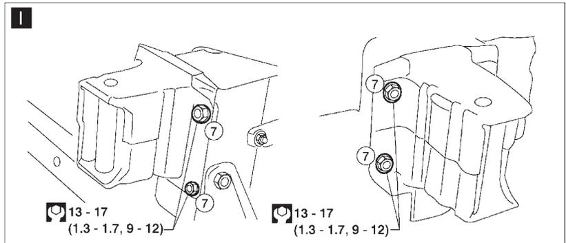
\* : Bumper assembly mounting bolts, screws, nuts, and clips
