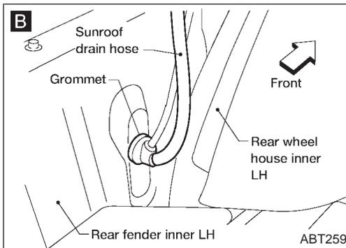
1. Remove headlining to access drain hose connections. (Refer to "REMOVAL — Headlining" in "INTERIOR TRIM", BT-25, for details.)
