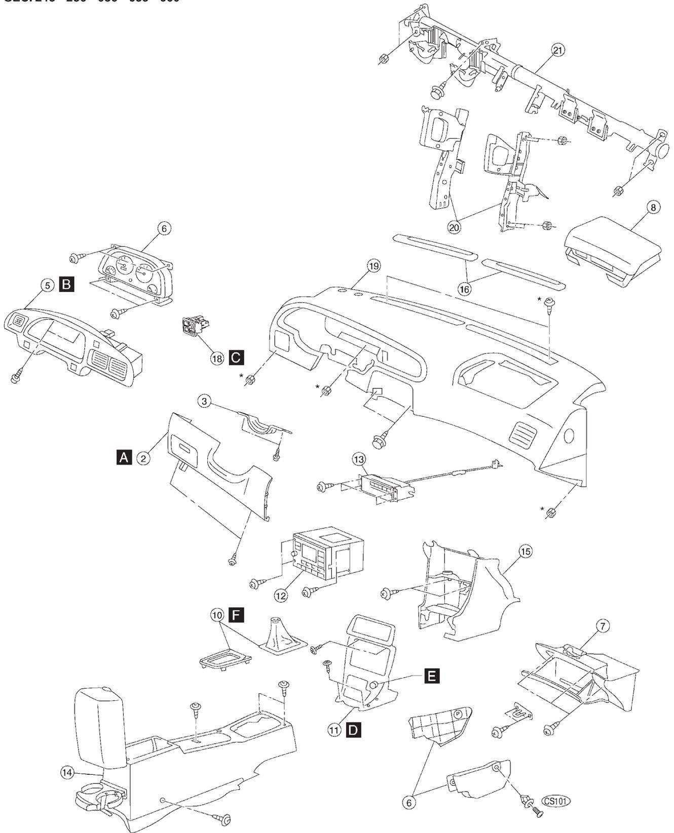
\* : Instrument panel assembly mounting bolts, screws and nuts.
