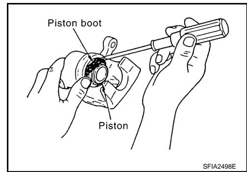
3. Apply brake fluid to piston. Push piston into cylinder body by hand and push piston boot piston side lip into the piston groove.
