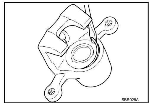
4. Place a wooden block as shown in the figure, and blow air from union bolt mounting hole to remove piston and piston boot.
