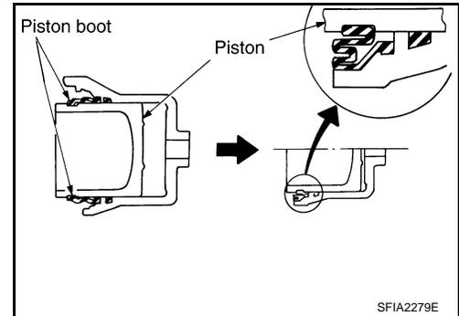
4. Secure piston boot with retaining ring.
