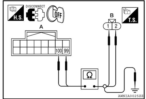
3. Check continuity between IPDM E/R harness connector E201 (A) terminals 99, 100 and ground.
