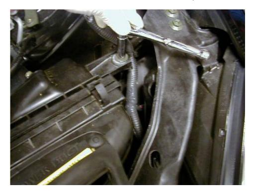
Then you can push the back side of the box backward and the front side forward to remove the filter. It's tight but it can be done.
