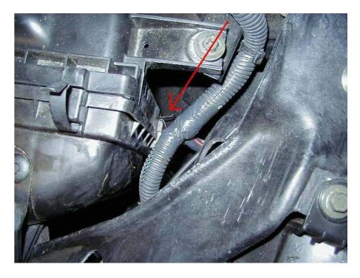
Remove the 10MM bolt that holds the back side of the air box to the body.
