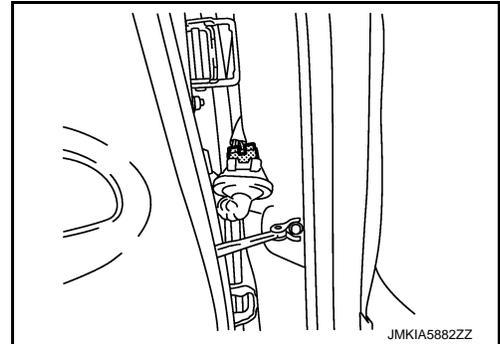
3. Remove mounting bolt of door check link on the vehicle.
