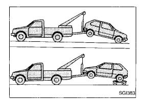
NISSAN recommends that vehicle be towed with the driving (rear) <sup>BT</sup> wheels off the ground as illustrated.
