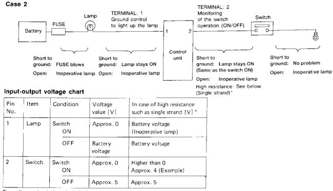
The voltage value is based on the body ground
