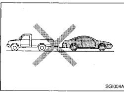
Never tow from the rear (i.e., backward) with four wheels on the ground as this may cause serious and expensive damage to the transmission.
