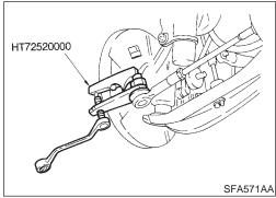
2. Remove tie-rod ball joint and lower ball joint.
