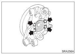
Remove wheel bearing with flange, and wheel hub from axle housing.
