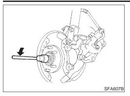
. Remove wheel bearing lock nut. Remove wheel hub from spindle.
