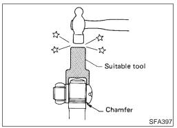
2. Install spider assembly securely, making sure marks are properly aligned.
