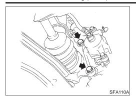
3. Remove brake caliper assembly and rotor.
