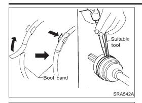
Lock new larger and smaller boot bands securely with a suitable tool.
