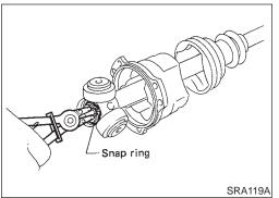
Pry off snap ring, then remove spider assembly.
