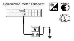
Higher rpm = Higher voltage Lower rpm = Lower voltage Voltage should change with rpm.
