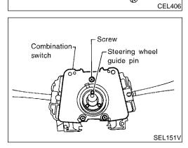
Before installing the steering wheel, align the steering wheel guide pins with the screws which secure the combination switch as shown in the left figure.
