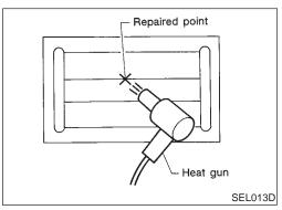
5. Apply a constant stream of hot air directly to the repaired area for approximately 20 minutes with a heat gun. A minimum distance of 3 cm (1.2 in) should be kept between repaired area and hot air outlet. If a heat gun is not available, let the repaired area dry for 24 hours.
