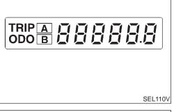
6. All odo/trip meter segments should be turned on.
