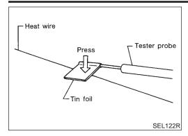
When measuring continuity, wrap tin foil around the top of probe. Then press the foil against the wire with your finger.
