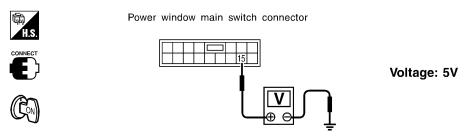
NOTE: Check voltage when power window regulator harness connector is disconnected.
