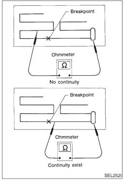
2. To locate broken point, move probe along element. Tester needle will swing abruptly when probe passes the point.
