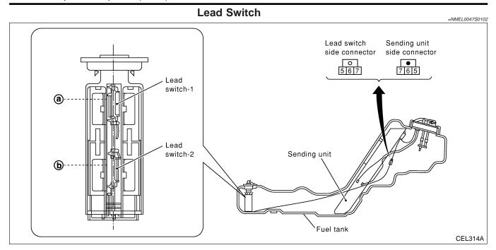
Lead switch is built into the fuel tank. Check the continuity between terminals 5 and 6 or 5 and 7.
