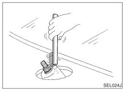
Before reinstalling wiper arm, clean up the pivot area as illustrated. This will reduce possibility of wiper arm looseness.
