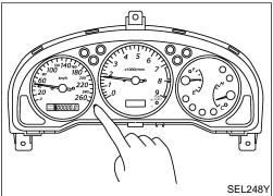
7. Push odo/trip meter switch. Indication of each meter/gauge should be as shown left during pushing odo/trip meter switch if it is no malfunctioning.
