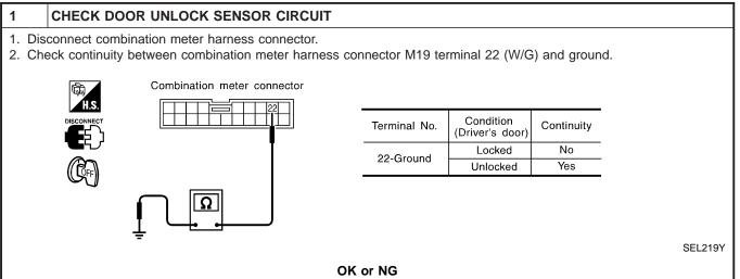
Door unlock sensor is OK; go to unified meter control unit (time control system) check. Refer to EL-133. NG GO TO 2. **CHECK DOOR UNLOCK SENSOR** 1. Disconnect door unlock sensor harness connector. 2. Check continuity between door unlock sensor harness connector D8 terminals 1 and 2.
