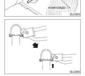
• Grip the crimped edge and bend it upwards so that Tool slips off.
