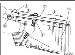
4. Caulk tank in specified sequence with Tool.
