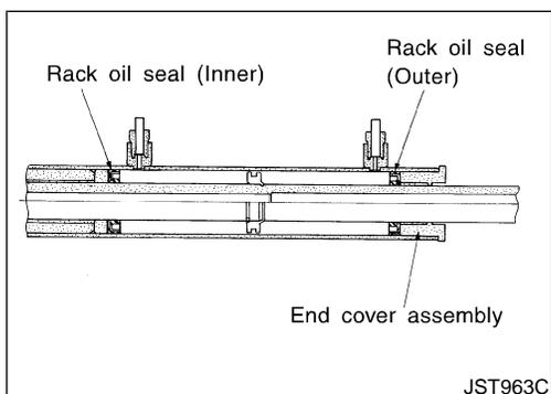
7. Install the inner and outer rack oil seal with both lips facing each other.
