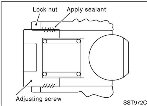
14. Install adjusting screw temporarily.
