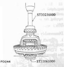
Fig. PD-14 Installing side bearing cone
