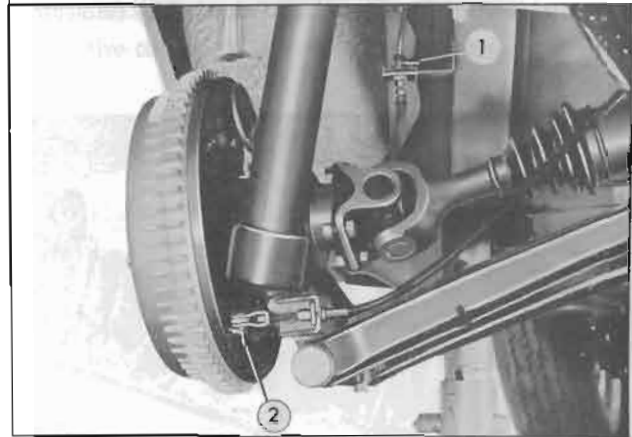
Fig. RA-10 Removing the brake hose and side brake linkage
