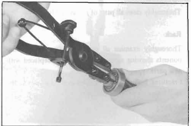
Fig. ST-22 Removing snap ring
