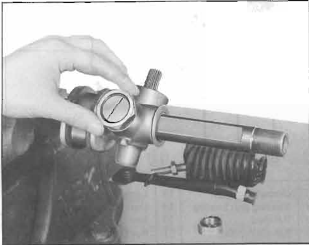
Fig. ST-18 Removing side rod outer socket
