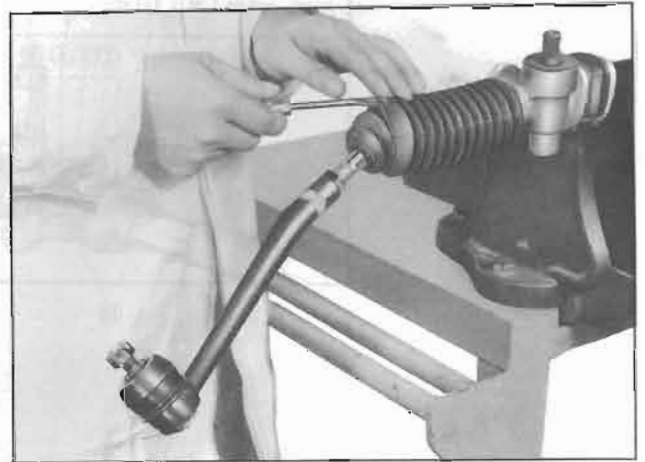
Fig. ST-16 Removing dust cover clamp
