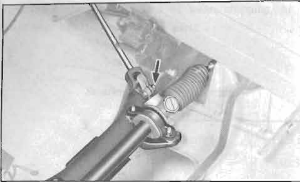
Fig. ST-13 Disconnecting lower joint from pinion
