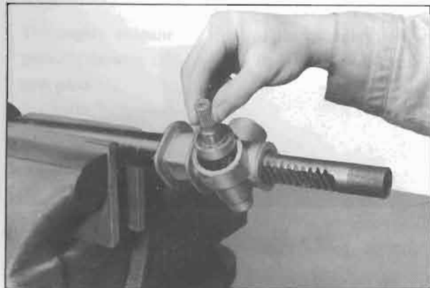
Fig. ST-27 Inserting pinion
