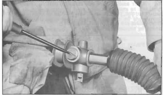
Fig. ST-32 Threading in adjusting screw
