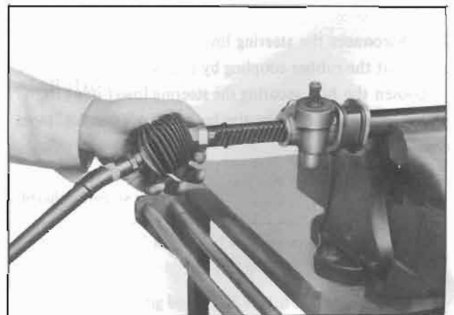
Fig. ST-17 Removing side rod assembly
