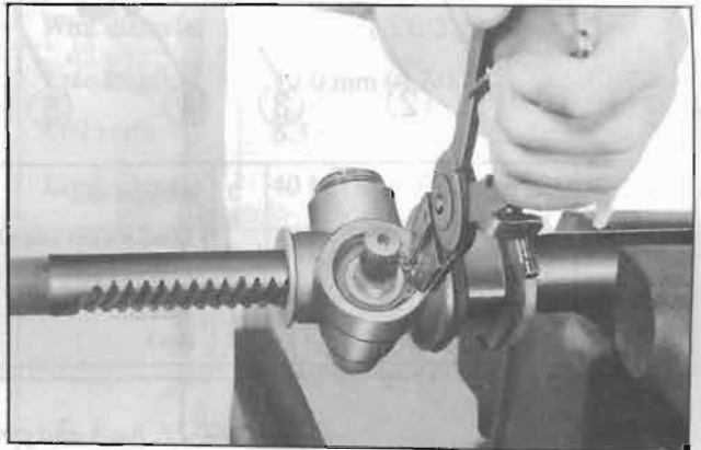
Fig. ST-21 Removing snap ring
