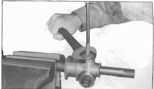
Fig. ST-33 Locking retainer lock nut
