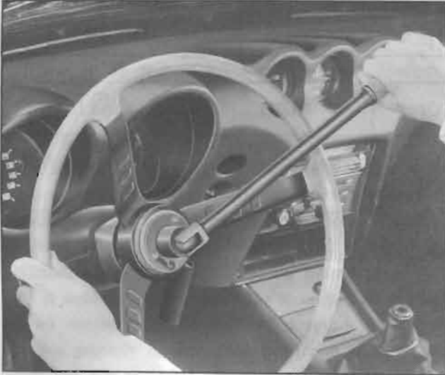
Fig. ST-3 Removing steering wheel
