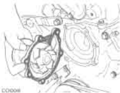
Fig. CO-3 Removing water pump
