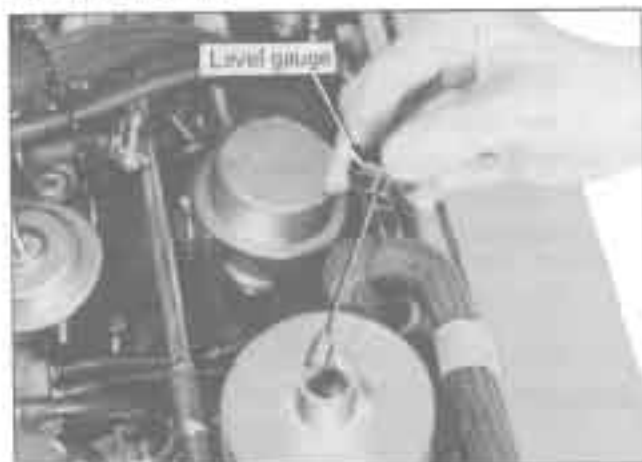
Fig. EF-32 Checking damper oil level
