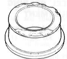
c) Cracked inner race
