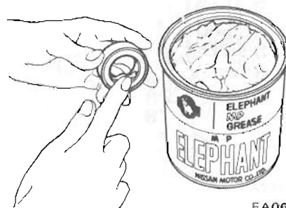
Fig. FA-23 Filling grease seal lip pocket with grease
