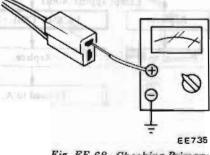
Fig. EE-68 Checking Primary Circuit 5. Turn ignition switch to "OFF" position.
