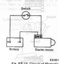
Fig. EE-19 Circuit of Magnetic Switch Assembly Test
