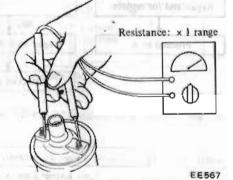
Fig. EE-69 Checking Ignition Coil Assembly
