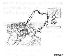
Fig. EE-41 Inspecting Sub-diode
