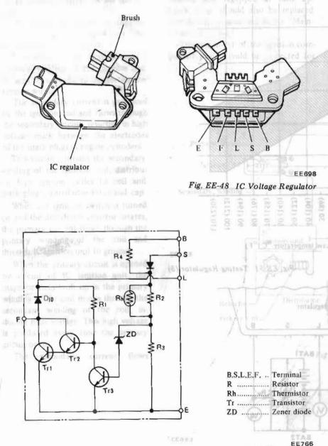
Fig. EE-49 Circuit of Regulator
