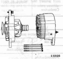
Fig. EE-26 Separating Front Cover
