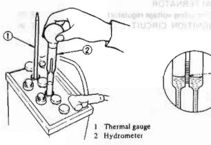
The gravity of electrolyte changes 0.0007 for every 1°C (1.8°F) temperature. Converted specific gravity at 20°C (68°F) can then be made by using the following formula:
