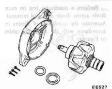
Fig. EE-28 Removing Rotor
