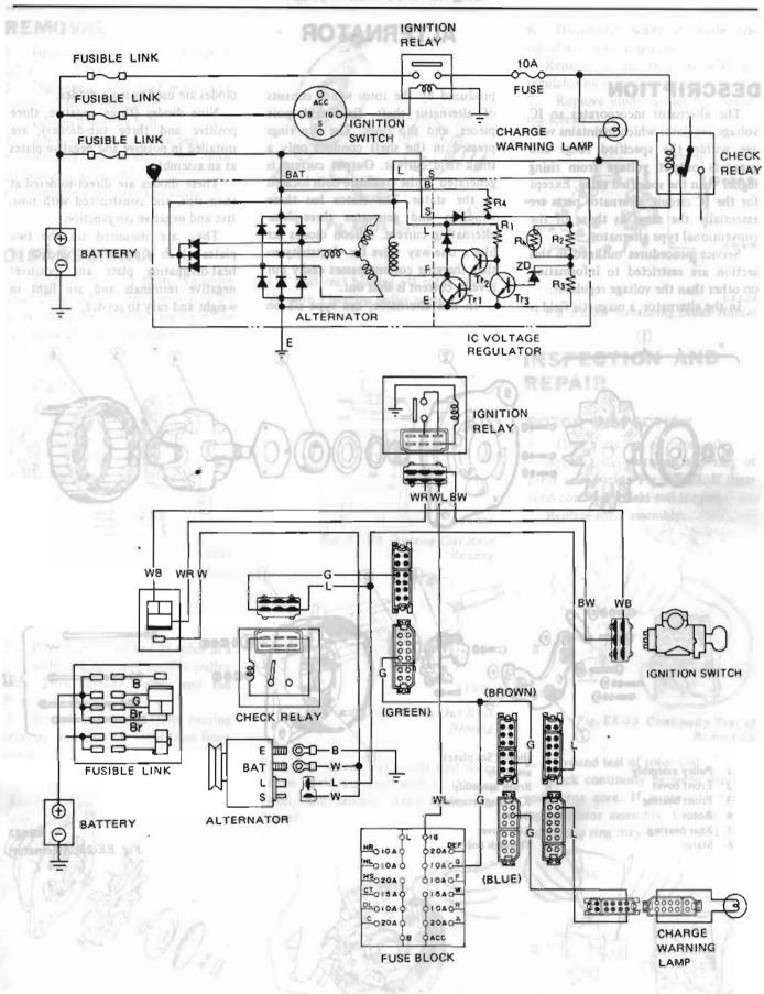
EE756 Fig. EE-24 Circuit Diagram of Charging System
