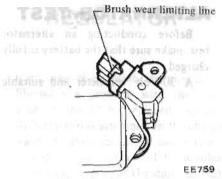
Fig. EE-43 Brush Wear Limit
