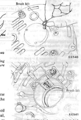
Fig. EE-46 Inserting Brush Lift
