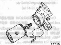
Fig. EE-7 Removing Yoke and Armature Assembly
