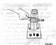
Fig. EE-15 Testing Armature for Short
