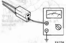
Fig. EE-67 Checking Power Supply Circuit
