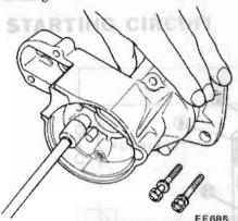
Fig. EE-9 Removing Center Housing
