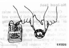
Fig. EE-17 Testing Brush for Ground
