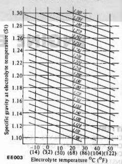
Fig. EE-3 Conversion of Specific Gravity
