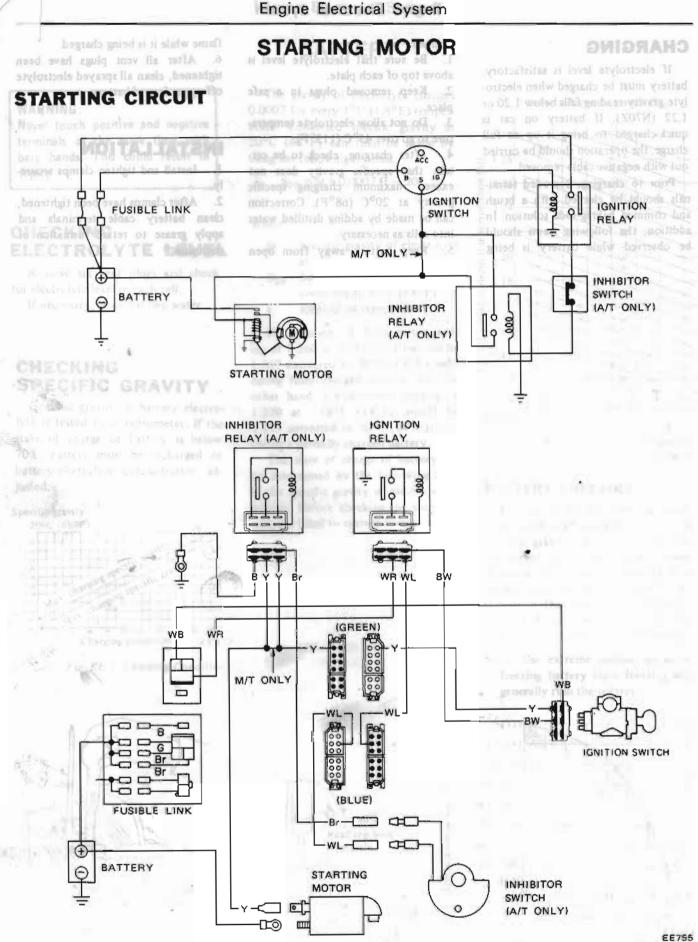
Fig. EE-5 Circuit Diagram of Starting System
