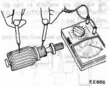
Fig. EE-14 Testing Armature for Ground
