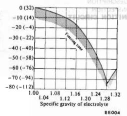
Fig. EE-2 Checking Specific Gravity
