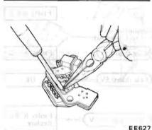
Fig. EE-42 Removing Sub-diode
