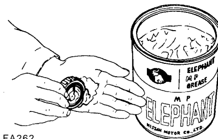
Fig. FA-20 Filling bearing cone with grease
