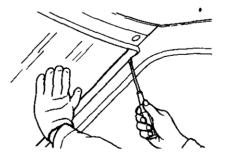
BF390A Fig. BF-57 Removing front windshield glass
