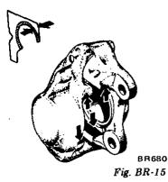
4. Install pad and anti-squeal shim, assemble anti-squeal spring and retaining pin, and secure them with clip.
