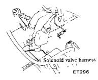
Fig. ET-26 Removing harness of solenoid valve
