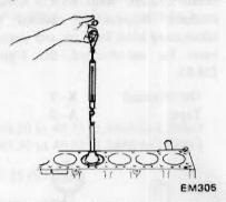
Fig. EM-56 Measuring piston fit in cylinder
