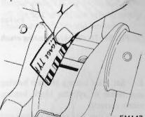
Fig. EM-69 Measuring bearing clearance
