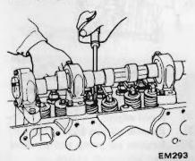
Fig. EM-31 Removing rocker arm
