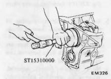
Fig. EM-94 Installing rear oil seal
