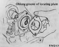
Fig. EM-83 Installing camshaft locating plate
