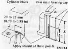
Fig. EM-79 Applying sealant
