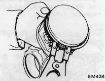
Fig. EM-29 Removing piston ring
