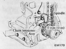
Fig. EM-102 Installing chain tensioner
