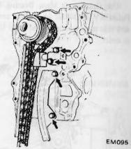
Fig. EM-22 Removing chain tensioner and timing chain
