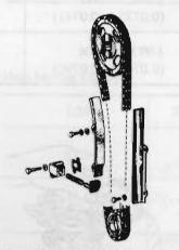
Fig. EM-75 Camshaft drive mechanism
