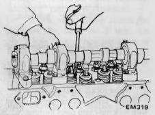
Fig. EM-85 Installing rocker arm
