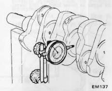
Fig. EM-64 Checking crankshaft bend
