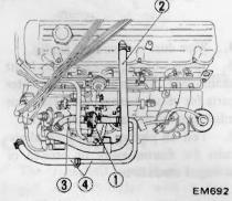
Fig. EM-10 Removing air regulator
