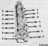
Fig. EM-100 Cylinder head bolts
