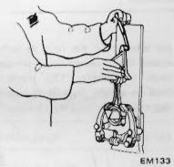
Fig. EM-61 Checking rod alignment
