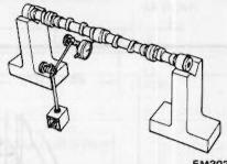
Fig. EM-50 Checking camshaft bend
