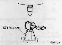
Fig. EM-87 Installing piston pin
