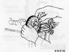
Fig. EM-72 Checking camshaft
