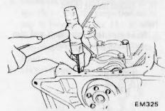
Fig. EM-93 Driving side oil seal
