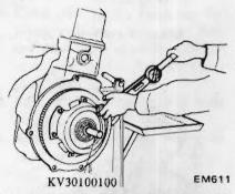
Fig. EM-112 Installing clutch assembly
