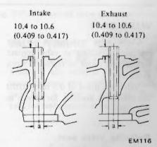
Fig. EM-43 Valve guide hole for service
