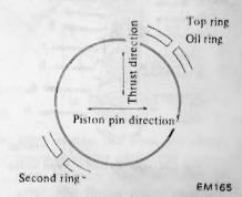
Fig. EM-97 Piston ring direction
