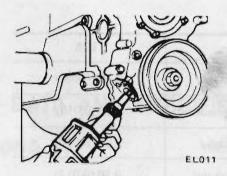
Fig. EM-108 Installing oil pump
