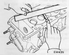
Fig. EM-35 Checking cylinder head surface
