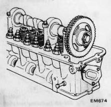
Fig. EM-86 Assembling cylinder head
