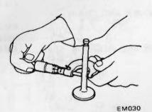
Fig. EM-37 Checking valve stem diameter
