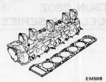
Fig. EM-4 Cylinder head
