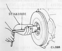
Fig. EM-66 Pulling out pilot bushing
