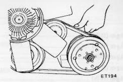
Fig. EM-114 Air conditioning compressor belt tension
