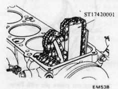
Fig. EM-19 Supporting timing chain
