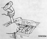
Fig. EM-92 Checking crankshaft end play
