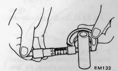
Fig. EM-60 Measuring piston pin diameter
