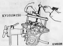
Fig. EM-26 Removing rear main bearing cap
