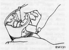
Fig. EM-59 Piston pin fitting
