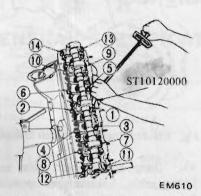
Fig. EM-106 Tightening sequence
