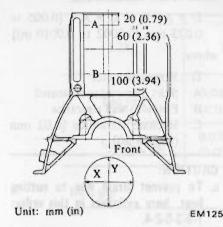
Fig. EM-53 Cylinder bore measuring positions
