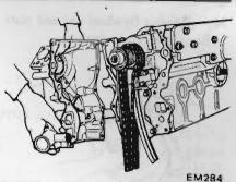
Fig. EM-21 Removing front cover
