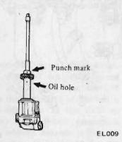
Fig. EM-107 Setting distributor driving spindle
