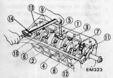
Fig. EM-91 Torque sequence of cap bolts
