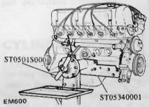
Fig. EM-9 Engine on engine stand
