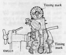
Fig. EM-103 Installing front cover
