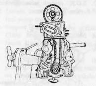
Fig. EM-7 Camshaft driving chain
