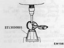
Fig. EM-30 Removing piston pin
