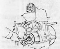
Fig. EM-105 Installing crankshaft pulley
