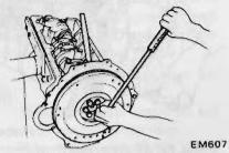
Fig. EM-25 Removing flywheel
