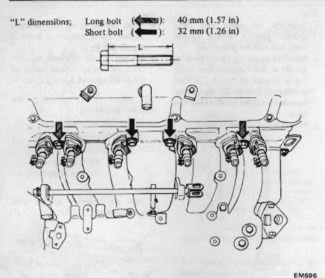
Fig. EM-111 Location of intake manifold securing bolts
