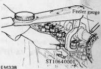
Fig. EM-110 Adjusting value clearance
