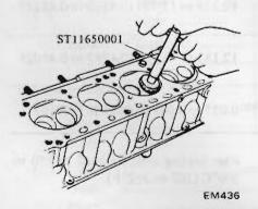
Fig. EM-45 Correcting valve seat
