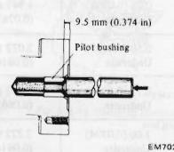
Fig. EM-67 Press-fitting new pilot bushing
