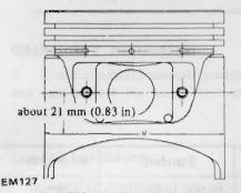
Fig. EM-55 Measuring piston skirt diameter
