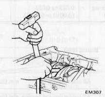
Fig. EM-65 Checking crankshaft end play
