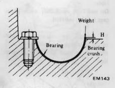
Fig. EM-70 Checking bearing crush
