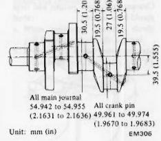
Fig. EM-63 Crankshaft and journal dimensions
