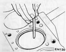
Fig. EM-58 Measuring ring gap
