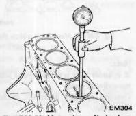
Fig. EM-52 Measuring cylinder bore diameter
