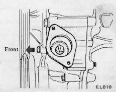
Fig. EM-109 Setting distributor drive spindle
