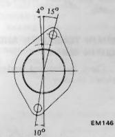
Fig. EM-73 Camshaft locate plate
