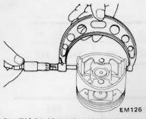
Fig. EM-54 Measuring piston diameter
