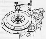
Fig. EM-76 Checking flywheel deviation
