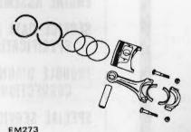
Fig. EM-3 Piston and connecting
