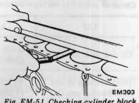
Fig. EM-51 Checking cylinder block surface
