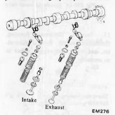
Fig. EM-6 Value mechanism
