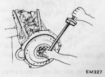
Fig. EM-95 Installing flywheel
