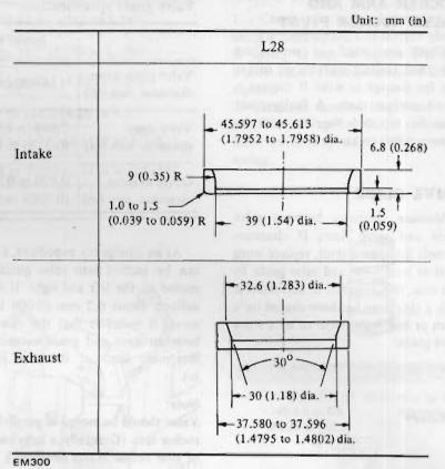
Fig. EM-46 Service valve seat dimensions
