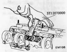
Fig. EM-33 Removing value
