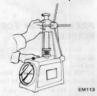
Fig. EM-40 Measuring spring tension
