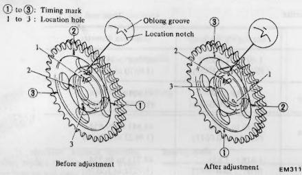
Fig. EM-74 Adjusting camshaft sprocket location
