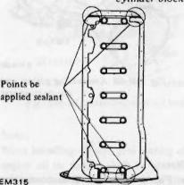
Fig. EM-80 Applying sealant (Cylinder block)
