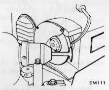
Fig. EM-38 Regrinding valve face
