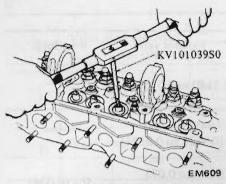
Fig. EM-44 Reaming valve guide
