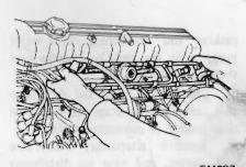
Fig. EM-13 Removing fuel pipe assembly
