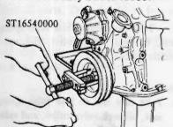
Fig. EM-18 Removing crank pulley
