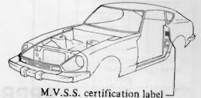
Fig. G1-6 M.V.S.S. certification label location
