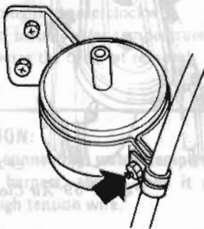
Fig. EF-61 Removing Fuel Filter
