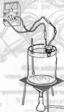
Fig. EF-120 Checking Water Temperature Sensing Switch
