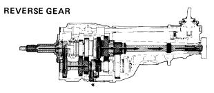
For reverse gear operation the reverse idler gear is moved to the rear, where it engages the reverse countershaft gear and the reverse sliding gear on the output shaft. The gears under power in reverse are input shaft, countershaft drive gear, reverse countershaft gear, reverse idler gear, reverse sliding gear, and output shaft.
