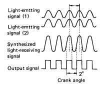
Signal used to detect the crank angle
