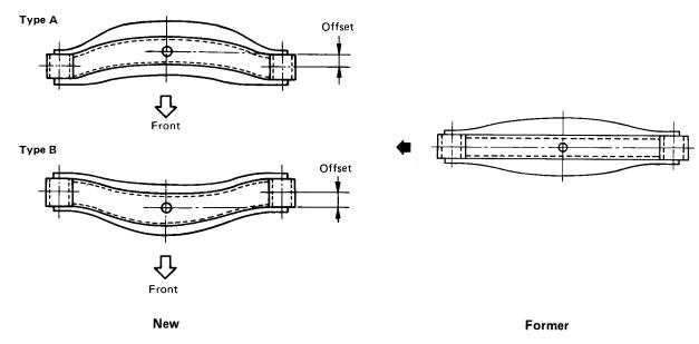
Type A: Models equipped with FS5R90A (Borg-Warner T-5) transmission
