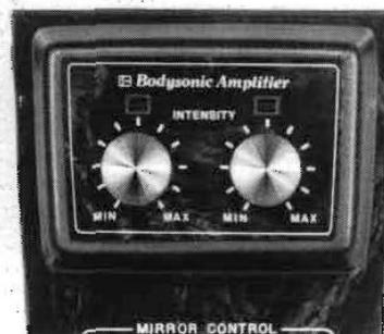
The controller permits independent adjustment of vibration intensity for the driver's seat and passenger seat. If the intensity control knob is pressed when the radio is ON, the internal switch of the controller turns ON, and the indicator lights up. Thus, the intensity can be adjusted by turning the control knob.
