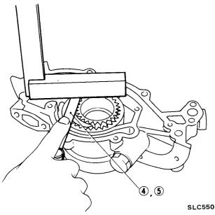
If excessive wear is found, replace gear set or entire oil pump assembly.
