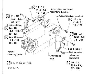
After installing oil pump, adjust belt tension.
