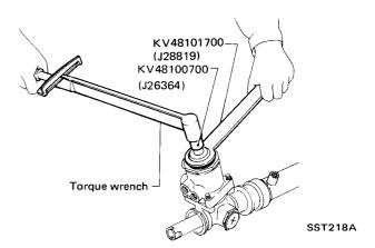
Pinion starting torque T<sub>1</sub>: Less than 0.7 N·m (7 kg-cm, 6.1 in-lb)
