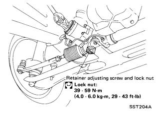
c) After adjustment, drive vehicle at low speeds to check for proper operation of steering system.
