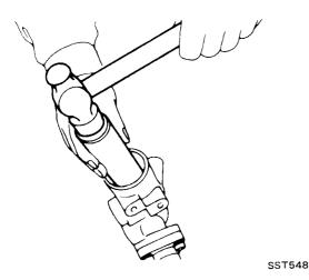
When installing cylinder end housing or rear housing cover, wrap cellophane tape around rack end or pinion serrations to prevent oil seal
