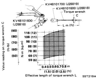
3. Measure pinion starting torque T<sub>3</sub> to make sure it is within specified range.
