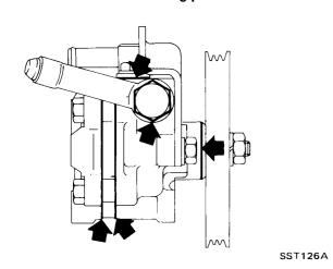
Deformed or damaged pulley
