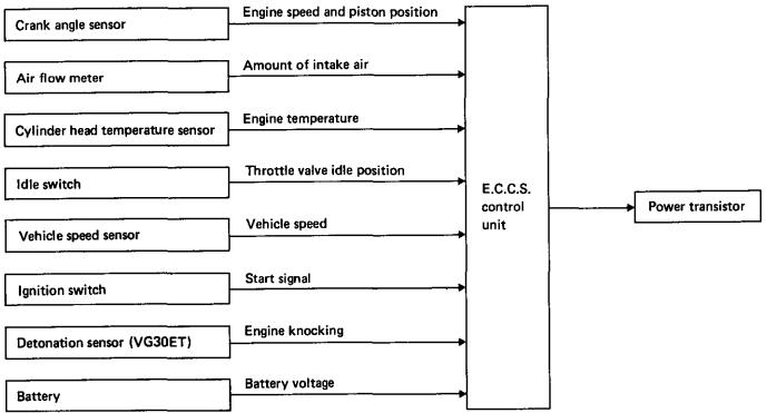
Ignition timing is controlled, corresponding to the engine operating conditions, by the E.C.U.: that is, as the optimum ignition timing in each driving condition has been pre-programmed in the control unit, the ignition timing is determined by electrical signals processed in the unit.
