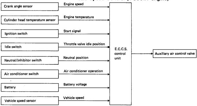
The idle speed is controlled by the E.C.U., corresponding to the engine operating conditions. The E.C.U. senses the engine condition and determines the best idle speed at each cylinder head temperature and gear position. The control unit then sends an electronic signal corresponding to the difference between the best idle speed and the actual idle speed to the A.A.C. valve.
