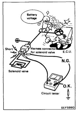
7. When measuring supply voltage of E.C.U. controlled components with a circuit tester, separate one tester probe from the other.
