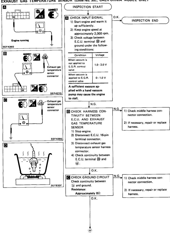
EXHAUST GAS TEMPERATURE SENSOR (Code No. 35); CALIFORNIA MODEL ONLY
