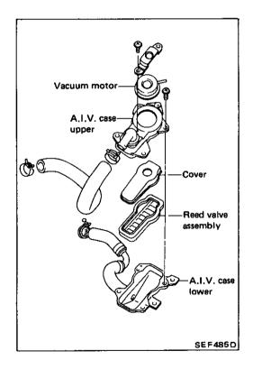
4. If the inspection shows N.G., disassemble the A.I.V. case and check such parts as the reed valve, the vacuum motor, and the connecting hoses.
