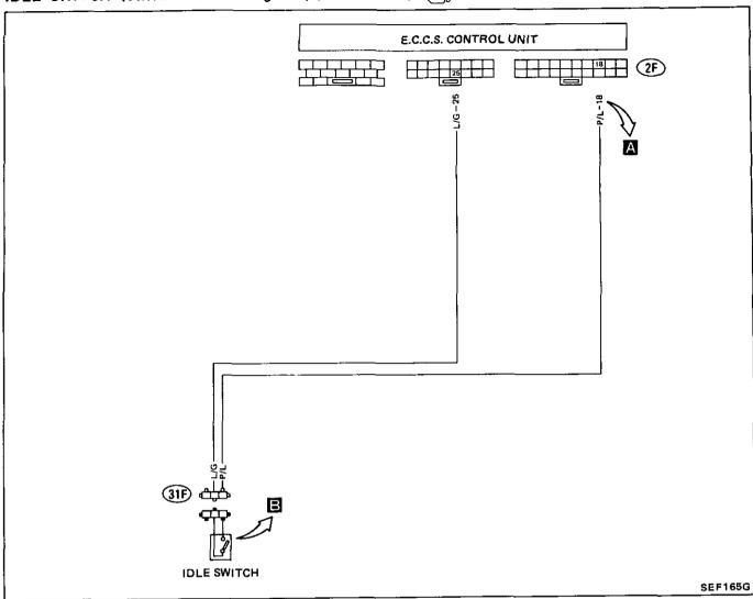
IDLE SWITCH (Switch ON/OFF diagnosis) (Code No. 23)
