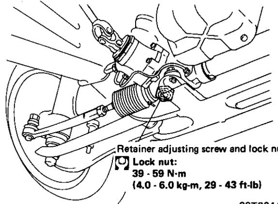
Retainer adjusting screw and lock nut
