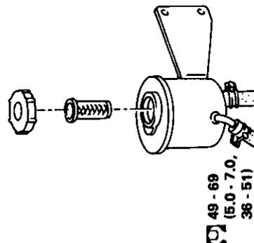
Oil pressure switch (Non-turbocharged model)
