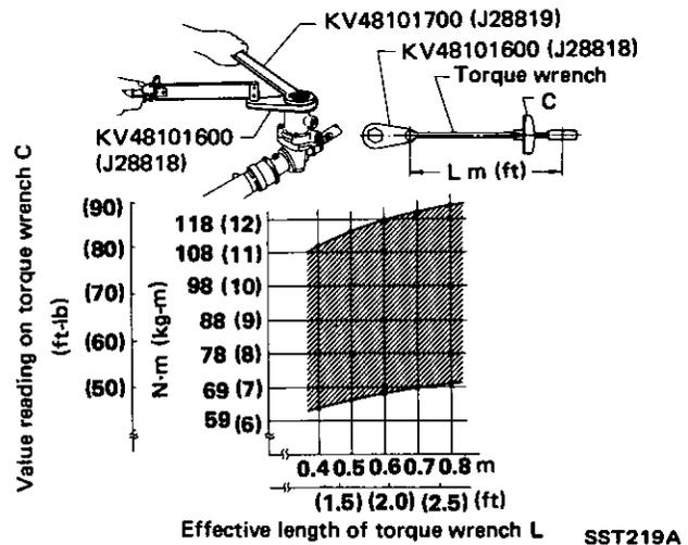
3. Measure pinion starting torque  $T_3$  to make sure it is within specified range.
