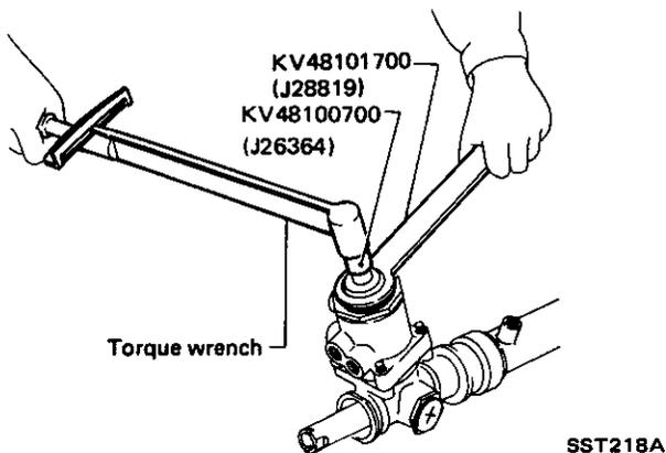
Pinion starting torque  $T_1$  :
