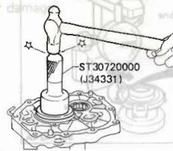
Counter gear rear bearing in adapter plate
