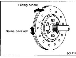
Check clutch disc for spline backlash and facing runout.
