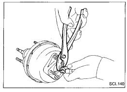
If amount of adjustment required exceeds 0.5 mm (0.020 in), reaction disc may have either been dislocated or fallen off. Replace clutch booster assembly.
