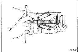
Install release bearing with suitable drift.
