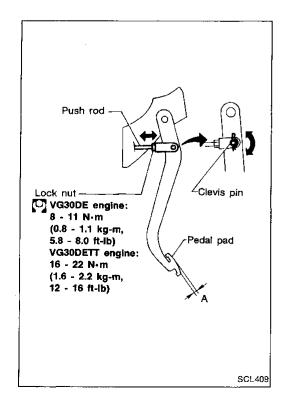
Adjust pedal free play with master cylinder push rod. Then tighten lock nut.
