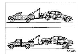
NISSAN recommends that vehicle be towed with the driving (rear) wheels off the ground as illustrated.
