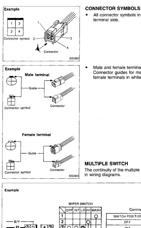
All connector symbols in wiring diagrams are shown from the
