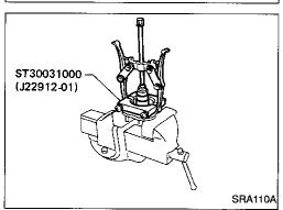
Remove inner race from hub using a bearing replacer/puller.
