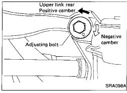
If camber is not within specification, adjust by turning the adjusting bolt.
