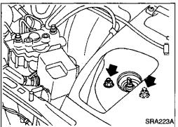
Remove upper end nuts of shock absorber.
