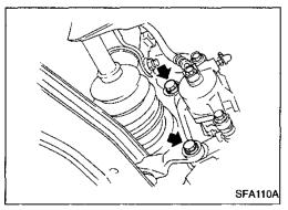
Remove brake caliper assembly.
