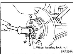
Separate drive shaft from axle housing by slightly tapping it. When removing drive shaft, cover boots with shop towel to prevent them from being damaged.
