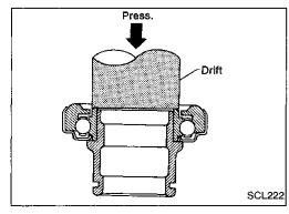
Install release bearing with suitable drift.
