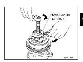
Remove the snap ring using external snap ring pliers.
