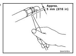
2. When testing, circle each fitting completely with probe.
