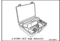
Position probe approximately 5 mm (3/16 in) away from point to be checked.
