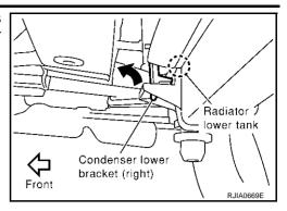
13. Pull condenser forward at an angle. Remove condenser from radiator.
