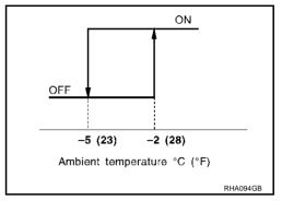
When intake air temperatures are greater than 1°C (34°F), the compressor turns ON. The compressor turns OFF when intake air temperatures are less than -5°C (23°F).
