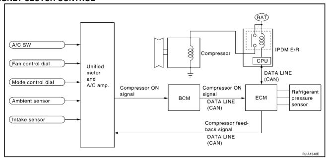
When A/C switch is pressed, turn fan control dial to ON or set mode control dial to D/F, D/F2 or DEF position, unified meter and A/C amp. (auto amp.) inputs compressor ON signal to BCM.
