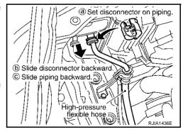
5. Remove the mounting nut for high-pressure flexible hose, and then remove the high-pressure flexible hose.
