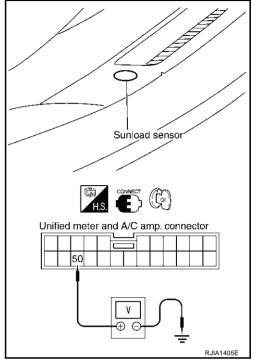
When checking sunload sensor, select a place where sun shines directly on it.
