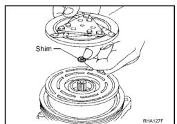
5. Using the holder to prevent clutch disc rotation, tighten the bolt to 14 N·m (1.4 kg·m, 10 ft - lb) torque.
