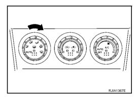
2. Confirm that discharge air comes out according to the air distribution table. Refer to <a href="ATC-33">ATC-33</a>, "Discharge Air Flow"</a>.
