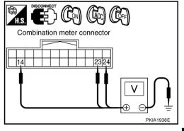
Check voltage between unified meter and A/C amp. connector and ground.
