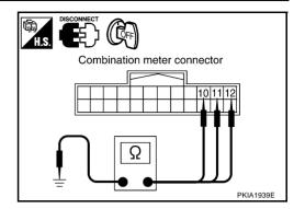
Check continuity between unified meter and A/C amp. and ground.
