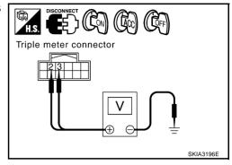
3. Check voltage between unified meter and A/C amp. harness connector terminals and ground.
