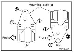
When reassembling main muffler only.
