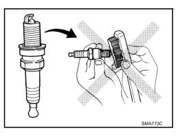
• Checking and adjusting plug gap is not required between change intervals.
