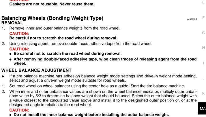
Before installing the balance weight, be sure to clean the mating surface of the road wheel.
