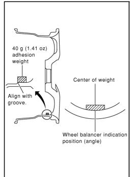
c. If calculated balance weight value exceeds 50 g (1.76 oz), install two balance weight sheets in line with each other (as shown in the figure).
