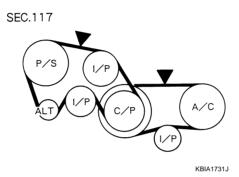
\*: If belt tension gauge cannot be installed at check points shown, check drive belt tension at different location on the belt.
