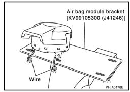
3. Connect deployment tool adapter [SST: J38381-80] to air bag module connector and deployment tool connector [SST: KV99106400(J38381)].
