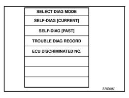
7. If no malfunction is detected on "SELF-DIAG [CURRENT]", repair of SRS is completed. Go to step 8. If any malfunction is detected on "SELF-DIAG [CURRENT]", the malfunctioning part is not repaired completely or another malfunctioning part is detected. Go to <a href="SRS-20">SRS-20</a>, "Diagnostic procedure 2", and repair malfunctioning part completely.
