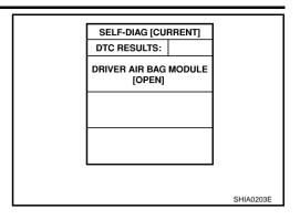
If no malfunction is detected on "SELF-DIAG [CURRENT]" even though malfunction is detected in "SRS Operation Check", check the battery voltage. If the battery voltage is less than 9V, charge or replace the battery. SRS-23, "DIAGNOSTIC PROCEDURE 3". If the battery voltage is OK, go to SRS-26, "DIAGNOSTIC PROCEDURE 4 (CONTINUED FROM DIAGNOSTIC PROCEDURE 2)" diagnose the following cases:
