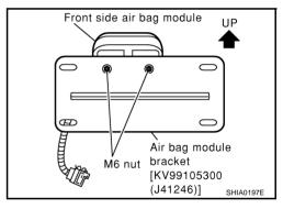
Connect deployment tool adapter [SST: KV99108300(J38381-35)] and deployment tool [SST: KV99106400 (J38381)] on side air bag module.
