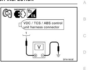
**VDC/TCS/ABS** control unit Ground **Signal name Measured value** (Harness connector E118) BRC **Power supply** 1 (G/R) Battery voltage (Approx. 12V) (OFF VDC / TCS / ABS control unit harness connector 28,29 Н Ω SFIA1897E **VDC/TCS/ABS** control unit **Signal name** Ground **Measured value** (Harness connector E118) 28 (B) Continuity should exist. Κ Ground 29 (B) Continuity should exist. \_\_\_\_ L
