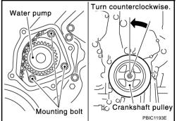
Screw M8 bolts [pitch: 1.25 mm (0.049 in) length: approx. 50 b. mm (1.97 in)] into water pumps upper and lower mounting bolt holes until they reach timing chain case. Then, alternately tighten each bolt for a half turn, and pull out water pump.
