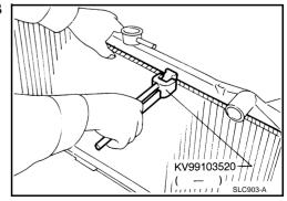
Grip the crimped edge and bend it upwards so that radiator plate pliers B slips off.
