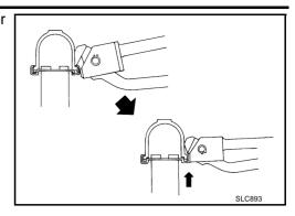
In areas where radiator plate pliers B cannot be used, use flat-blade screwdriver to bend the edge up.
