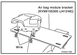
3. Connect deployment tool adapter (SST: J38381-80) to air bag module connector and deployment tool connector [SST: KV99106400 (J38381)].
