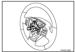
7. Loosen the spiral cable fixing screws, remove the spiral cable.
