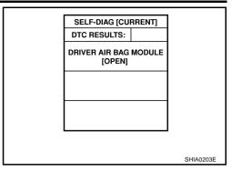
If no malfunction is detected on "SELF-DIAG [CURRENT]" even though malfunction is detected in "SRS Operation Check", check the battery voltage. If the battery voltage is less than 9 V, charge or replace the battery. <u>SRS-28</u>, "<u>DIAGNOSTIC PROCEDURE 3</u>". If the battery voltage is OK, go to <u>SRS-30</u>, "<u>DIAGNOSTIC PROCEDURE</u> 4 (CONTINUED FROM DIAGNOSTIC PROCEDURE 2)" diagnose the following cases:
