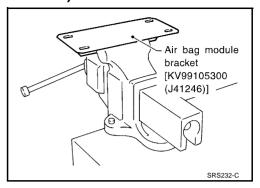
2. Match the hole in air bag module bracket (held in vise) and front passenger air bag module and fix them with one bolt  $[M8 \times 25 - 30 \text{ mm} (0.98 - 1.18 \text{ in})]$ .
