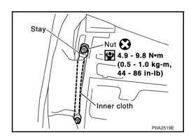
Remove the front side air bag module.
