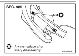
5. Remove the front side air bag module.
