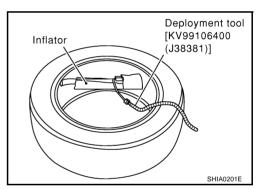
4. Put the tire with the inflator onto another tire without wheel. Add an additional tire without a wheel and then a tire mounted on a wheel on top.
