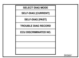
7. If no malfunction is detected on "SELF-DIAG [CURRENT]", repair of SRS is completed. Go to step 8. If any malfunction is detected on "SELF-DIAG [CURRENT]", the malfunctioning part is not repaired completely or another malfunctioning part is detected. Go to <u>SRS-24</u>, "<u>DIAGNOSTIC PROCEDURE 2</u>", and repair malfunctioning part completely.
