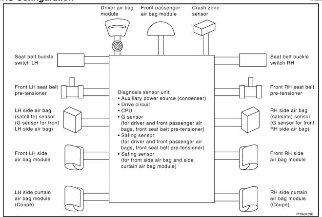
The air bag deploys if the diagnosis sensor unit activates while the ignition switch is in the ON or START position.
