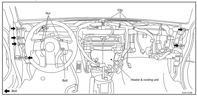
14. Remove heater & cooling unit.
