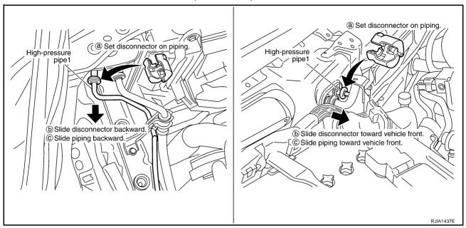
c. Slide A/C piping toward vehicle front (or backward) and disconnect it.
