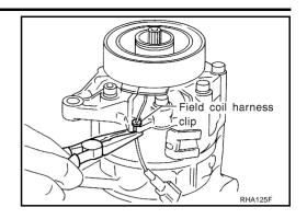
6. Remove snap ring using external snap ring pliers.
