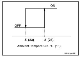
When intake air temperatures are higher than 1°C (34°F), the compressor turns ON. The compressor turns OFF when intake air temperatures are lower than -5°C (23°F).
