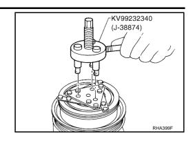
2. Remove clutch disc using clutch disc puller.
