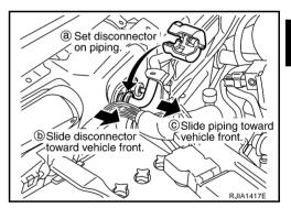
Remove mounting nut from low-pressure flexible hose. (Compressor side)
