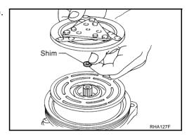
5. Using holder to prevent clutch disc rotation.
