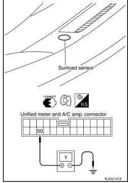
When checking sunload sensor, select a place where sun shines directly on it.
