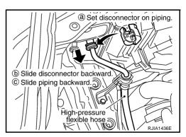
5. Remove mounting nut from high-pressure flexible hose, and then remove high-pressure flexible hose.
