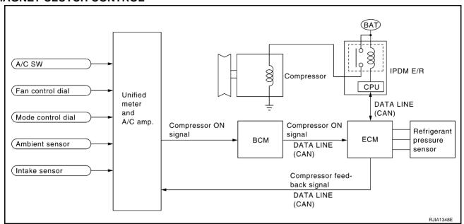
When A/C switch is pressed, turn fan control dial to ON or set mode control dial to D/F, D/F2 or DEF position, unified meter and A/C amp. inputs compressor ON signal to BCM.
