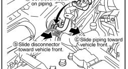
Remove clamps, and then disconnect two heater hoses from heater core.
