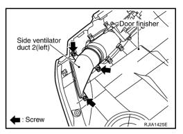
3. Remove mounting clips, and then remove side ventilator grille.
