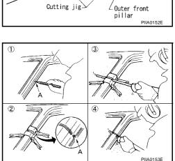
• Determine cutting position and record distance from the locating indent. Use this distance when cutting the service part. Cut outer front pillar over 60 mm above inner front pillar cut position.
