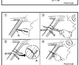
• Determine cutting position and record distance from the locating indent. Use this distance when cutting the service part. Cut outer front pillar over 60 mm above inner front pillar cut position.
