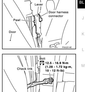
2. Remove the mounting bolts of the check link on the vehicle.
