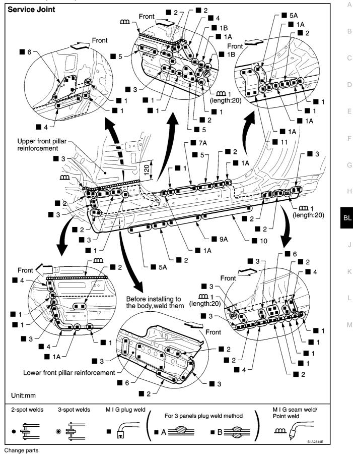
• Outer sill reinforcement assembly (LH) • Lower front pillar reinforcement (LH)
