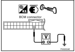
\*: When interior lamp battery saver control is in OFF position.  $\rightarrow$  Approx.5V
