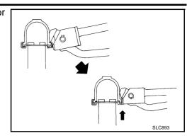
In areas where radiator plate pliers B cannot be used, use screwdriver to bend the edge up.
