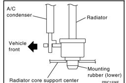
b. Lift A/C condenser up and remove radiator after disengaging the fitting as front-bottom surface.
