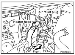
3. Fill radiator with water until water spills from the air relief hole, then close air relief plug. Fill radiator and reservoir tank with water and reinstall radiator cap.
