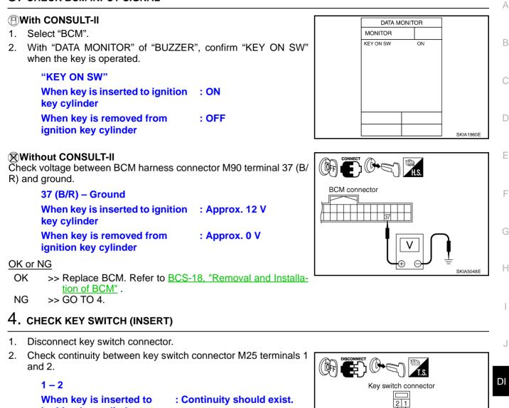
ignition key cylinder When key is removed : Continuity should not from ignition key cylinder exist.
