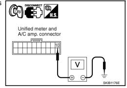
8. CHECK VOLTAGE SIGNAL OF UNIFIED METER AND A/C AMP.
