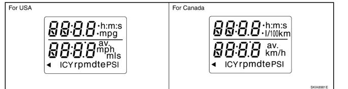
5. Push the odo/trip meter switch. Each meter/gauge should indicate as shown in the figure while pushing odo/trip meter switch.
