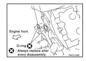
Install new O-rings to cylinder head.
