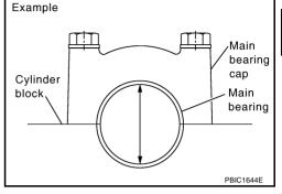
If the clearance exceeds the limit, select proper main bearing according to main bearing inner diameter and crankshaft main journal diameter to obtain the specified bearing oil clearance. Refer to <u>EM-154</u>, <u>"HOW TO SELECT MAIN BEARING"</u>.
