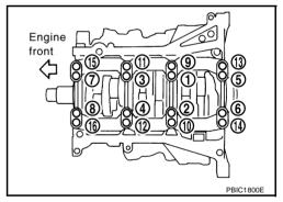
c. Turn all bolts another 90 to 95 degrees clockwise [Target: 90 degrees (Angle tightening)].
