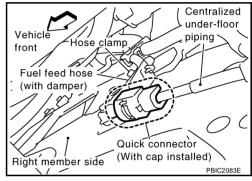
c. Disconnect quick connector from centralized under-floor piping as follows:
