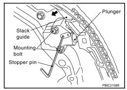
28. Remove internal chain guide, tension guide and slack guide.
