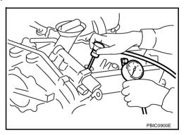
Use the adapter whose picking up end inserted to spark plug hole is smaller than 20 mm (0.79 in) in diameter. Otherwise, it may be caught by cylinder head during removal.
