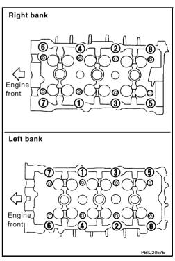
Turn all bolts 90 to 95 degrees clockwise [target: 90 degrees (angle tightening)].
