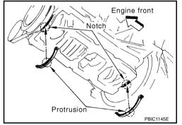
c. Install new O-rings on the bottom of cylinder block and oil pump.
