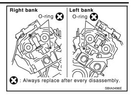
34. Remove O-rings from cylinder block.
