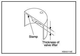
Available thickness of valve lifter: 27 sizes with range 7.88 to 8.40 mm (0.3102 to 0.3307 in) in steps of 0.02 mm (0.0008 in) (when manufactured at factory). Refer to <u>EM-171</u>, "Available <u>Valve Lifter"</u>.
