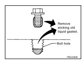
37. Use scraper to remove all traces of liquid gasket from water pump cover, chain tensioner cover and intake valve timing control covers.
