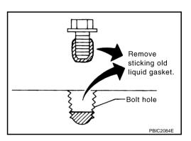
36. Use scraper to remove all traces of liquid gasket from water pump cover, chain tensioner cover and intake valve timing control covers.
