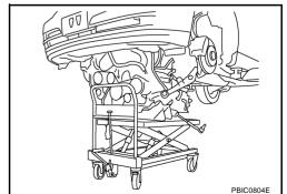
2. Remove rear engine mounting member bolts.
