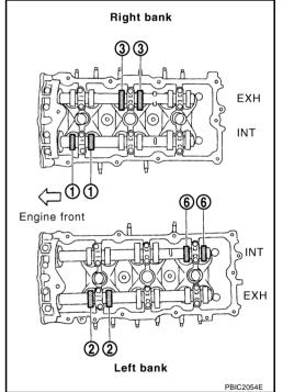
c. Rotate crankshaft by 240 degrees clockwise (when viewed from engine front) to align No. 3 cylinder at TDC of its compression stroke.
