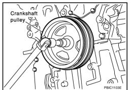
c. Place suitable puller tab on holes of crankshaft pulley, and pull crankshaft pulley through.
