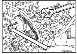
c. Remove timing chain (secondary) together with camshaft sprockets.
