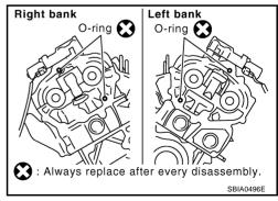
33. Remove O-rings from cylinder block.
