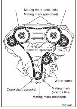
Install internal chain guide, slack guide and timing chain tensioner (primary).
