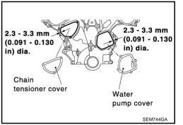
5. Install front timing chain case as follows:
