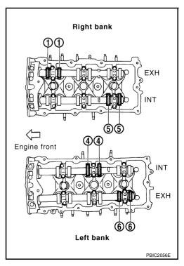
3. If the measured values are out of the standard, perform adjustment. Refer to EM-115, "ADJUSTMENT"
