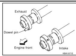
Follow your identification marks made during removal, or follow the identification marks that are present on new camshafts for proper placement and direction.
