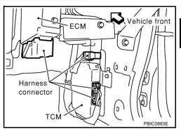
3. Disengage intermediate fixing point. Pull out engine room harnesses to engine room side, and temporarily secure them on engine.
