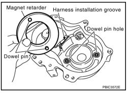
c. To check the joint between dowel pins and dowel pin holes, check the looseness in the axle direction by pushing the mating surface of magnet retarder at several places and the circumferential looseness (between dowel pins and dowel pin holes) by twisting in the circumferential direction.
