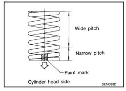
7. Install valve spring retainer.
