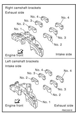
• Install camshaft brackets (No. 2 to 4) aligning the stamp marks as shown in the figure.
