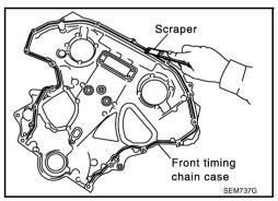
Remove old liquid gasket from bolt hole and thread.
