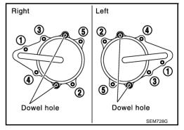
15. Remove left and right valve timing control covers (including magnet retarder and cover) with the following procedure. (For 35<sup>th</sup> Anniversary)
