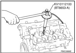
After installing cylinder head, measure distance between front end faces of cylinder block and cylinder head (left and right banks).
