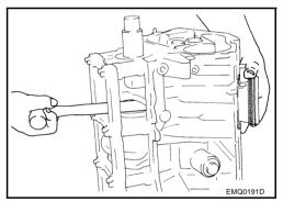
16. Remove connecting rod bearings from connecting rod and connecting rod bearing cap.
