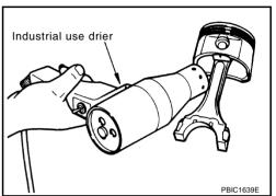
Push out piston pin with stick of outer diameter approximately 20 mm (0.79 in).
