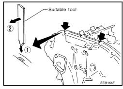
24. Remove O-rings from rear timing chain case.
