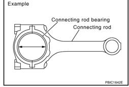
If the calculated value exceeds the limit, select proper connecting rod bearing according to connecting rod big end diameter and crankshaft pin journal diameter to obtain the specified bearing oil clearance. Refer to <u>EM-153</u>, "<u>HOW TO SELECT CONNECTING ROD BEARING</u>".
