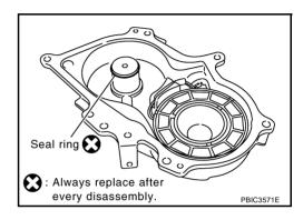
b. Install magnet retarder aligning the dowel pins of the back with the cover side dowel pin holes securely. Simultaneously insert the harness into the installation groove securely.
