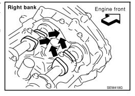
20. Remove crankshaft pulley as follows:
