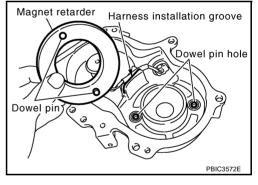
c. To check the joint between dowel pins and dowel pin holes, check the looseness in the axle direction by pushing the mating surface of magnet retarder at several places and the circumferential looseness (between dowel pins and dowel pin holes) by twisting in the circumferential direction.
