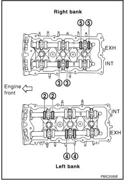
d. Rotate crankshaft by 240 degrees clockwise (when viewed from engine front) to align No. 5 cylinder at TDC of compression stroke.
